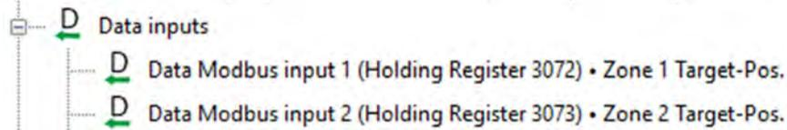
The data Modbus inputs are assigned to the respective ventilation link and set to the "target position" functionality.
