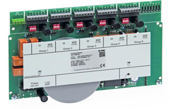
Control multiple drive groups at the same time: The GVL 8408-M control panel is our powerful variant for controlled natural ventilation.
