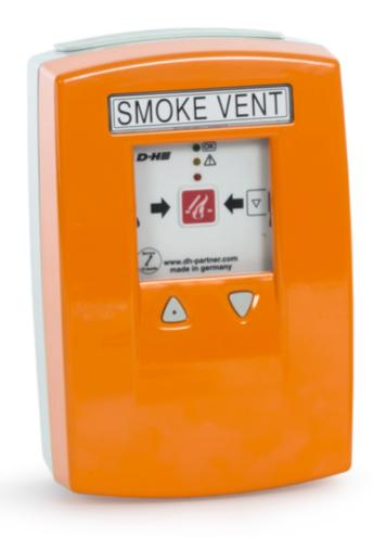
The SHEV control panel, ventilation button and trigger button are installed in one housing. The D+H control panel has an output of 3 A and is ideal for stairwells and single rooms. VdS certified according to ISO 21927-9, fulfils DIN 18232-9.
