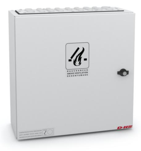
Pre-assembled SHEV control panel with 20 A load current. It is equipped with 6 combined RT and RM lines and 6 controllable motor connections. VdS certified according to ISO 21927-9, fulfils DIN 18232-9.
