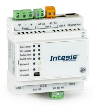
This allows D+H control panels and drives with ACB technology to be connected to BACnet-based building management systems. Programming using SCS software.
