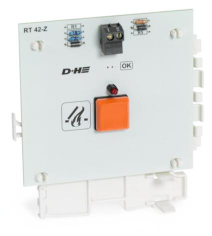
Reduced wiring effort: Our RT BE42-Z-K expansion operation unit requires only a two-wire cable for supply and communication.
