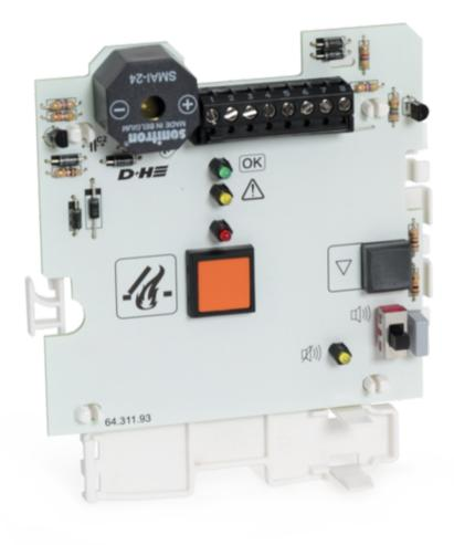
In addition to the operating lights for alarm, fault and monitoring, the SHEV operation unit RT BE42-ST has an additional acoustic signal emitter.
