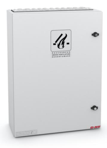
This CPS-M with a load current of 40 A, up to 6 combined RT & RM lines and 6 controllable motor connections ensures smoke and heat exhaust ventilation. VdS certified according to ISO 21927-9, fulfils DIN 18232-9.
